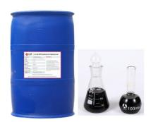
Film forming fluoro-protein foam concentrate (FFFP) consisting of hydrolysed protein and a blend of fluorocarbon-, hydrocarbon surfactants and various solvents and stabilisers. Only C6 Pure fluoro-surfactants are used in FFFP-formulations. FFFP 3% utilises the unique film forming effect to cut of oxygen supple to the fire and the oleophobic properties of the foam enables a stable foam blanket to suppress reignition of the fire.
